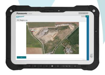
Airports may be required to monitor and record bird activity at nearby sites which, by attracting birds, could increase risk for the airport itself. Using a rugged tablet touch-screen pc, a built in GPS receiver and data collection software, Scarecrow's O.A.R software system creates a complete record of offsite activity and wildlife observations.
